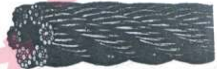
Right-hand Regular Lay (Ordinary Lay)
