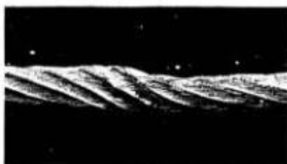
11. A KINK after straightening (note misplaced wires and strands). Also localised shortening of its length. This rope is now dangerous.
